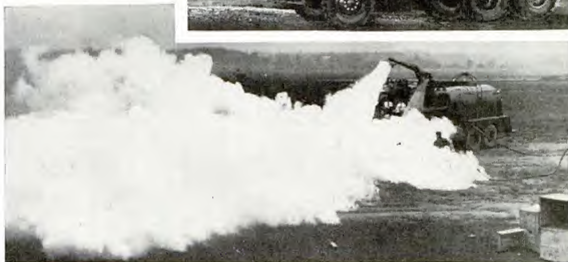
Approaching a burning plane, the truck sprays carbon dioxide from nozzles on front. Inset, control panel
